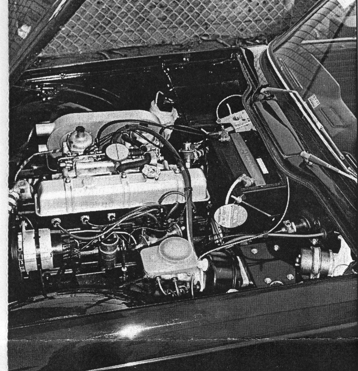
The stout heart of a TR6: Its 2.5-liter inline-6 proved to be easy to maintain and trouble-free. Beware careless clutch work, though. Backyard mechanics have been known to mismatch Borg & Beck and Laycock components.
