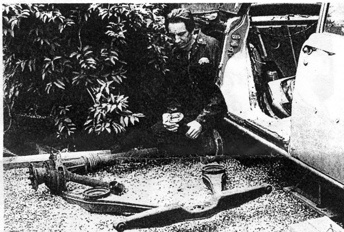
P6 rear suspension members are worth rescuing even though they are not easy to remove, because they do tend to corrode
