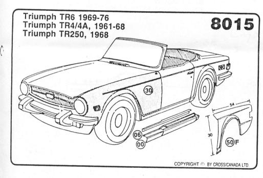
8015-00½ Rocker Panel, Compl. 8015-06½ Inner Rocker Panel Front Fender Fibreglass TR-6 Only
