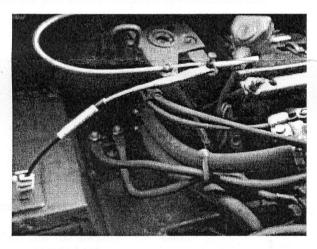
The original cable is the top looped cable directly connected to the hood latch release mechanism.
