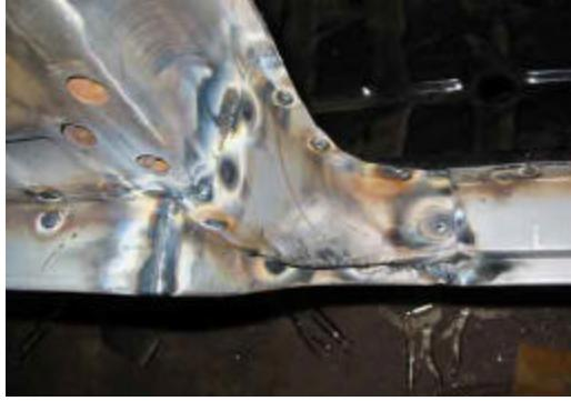
The welds had been ground off, using a 36 grid, flexible disk on a small air powered grinder.
