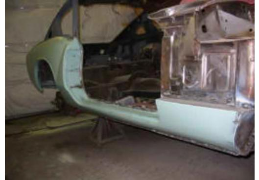
Prepping a repair in this fashion is crucial to a good paint job and should not be under estimated. One should not make the mistake of applying more body filler than absolutely necessary. It's important to realize that sanding off excess body filler is more important than applying more filler than needed. To protect the underside of the floor from stone chips, we sprayed an application of gravel guard.
