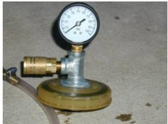
Next, you will need a spare cap off of an old master cylinder. Bore a hole in the center, use some blue silicon sealer to be sure you are airtight. Attach a standard pressure gauge to the t connector, use a quick connect on the other side. You get something like this:
