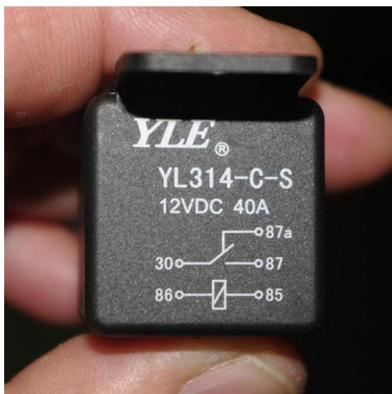
Figure 2. Relay showing configuration of terminals.
