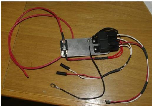
Figure 1. Breaker and relays.
