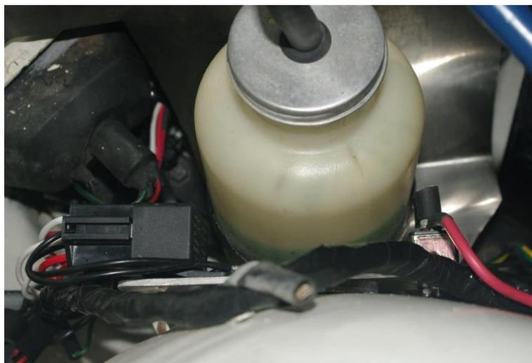
Figure 7. Final installation mounted to overflow bottle bracket.
