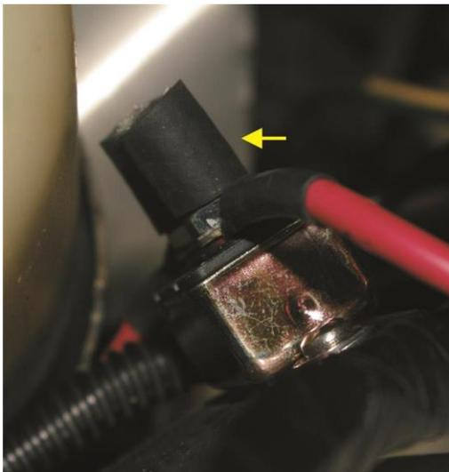
Figure 6. Terminals of circuit breaker insulated with short pieces of rubber hose.
