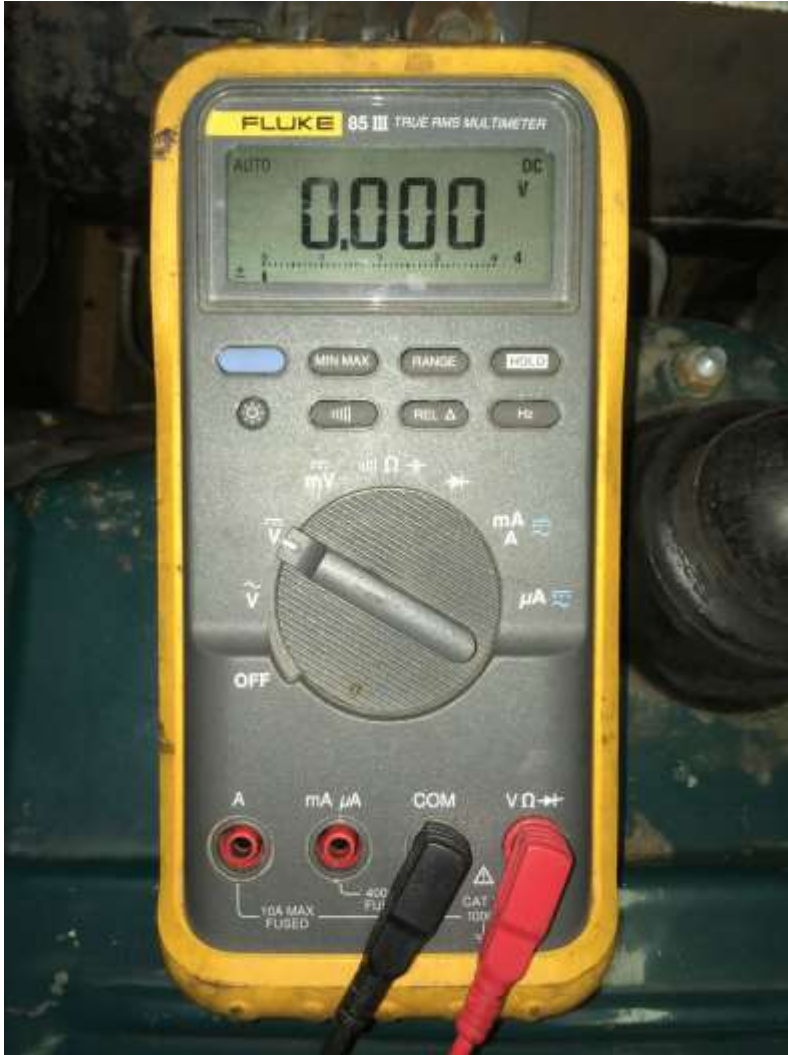
A multimeter configured to measure voltage (red probe in the “VR” socket, rotary dial turned to DC voltage setting).
