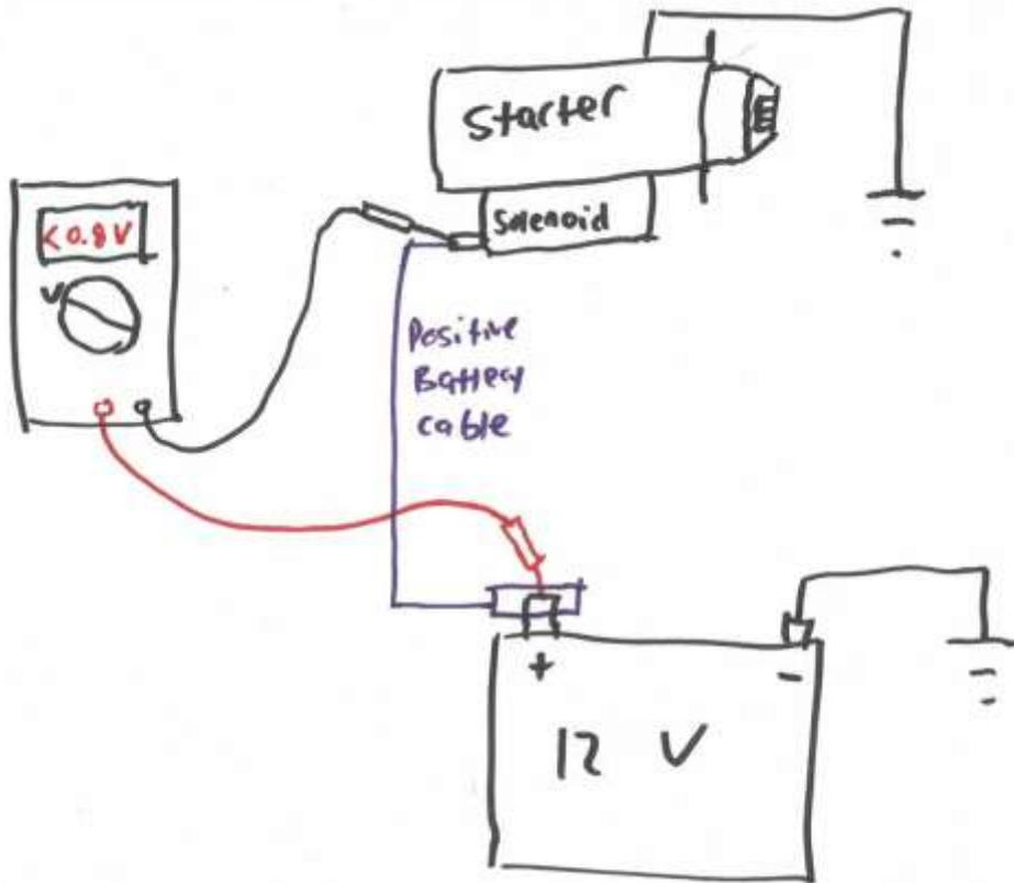
*The basics of a voltage drop measurement, where both probes of the meter are placed on the same side of the circuit (here, shown between the positive battery terminal and the positive post on the starter solenoid).*
