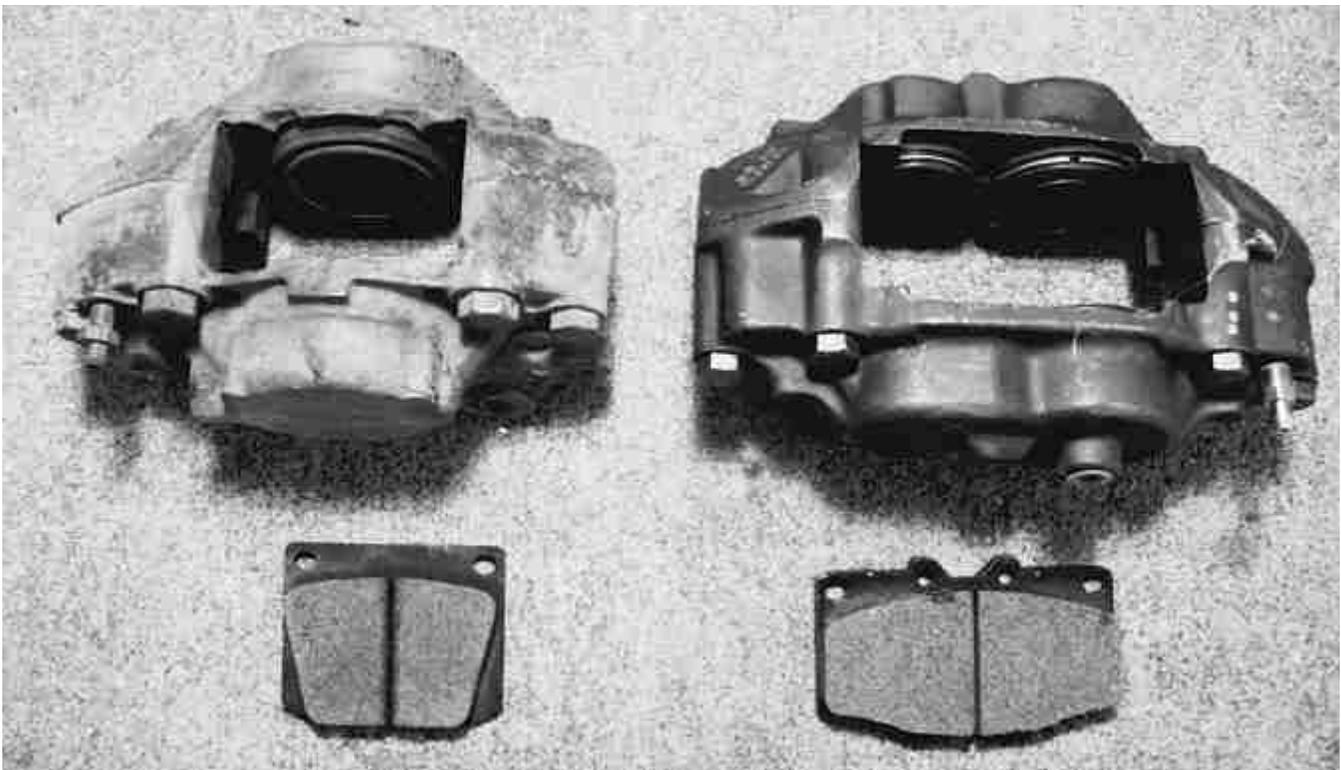
This illustrates the stock brake and pad on left and the Toyota on the right. The total lining area for the Toyota is approximately 27.8 in<sup>2</sup> or 179 cm<sup>2</sup>, a 34% increase over the lining area for the TR6. This increased area combined with the large size of the caliper may help reduce pad and caliper temperatures, and thereby reduce brake fade.
