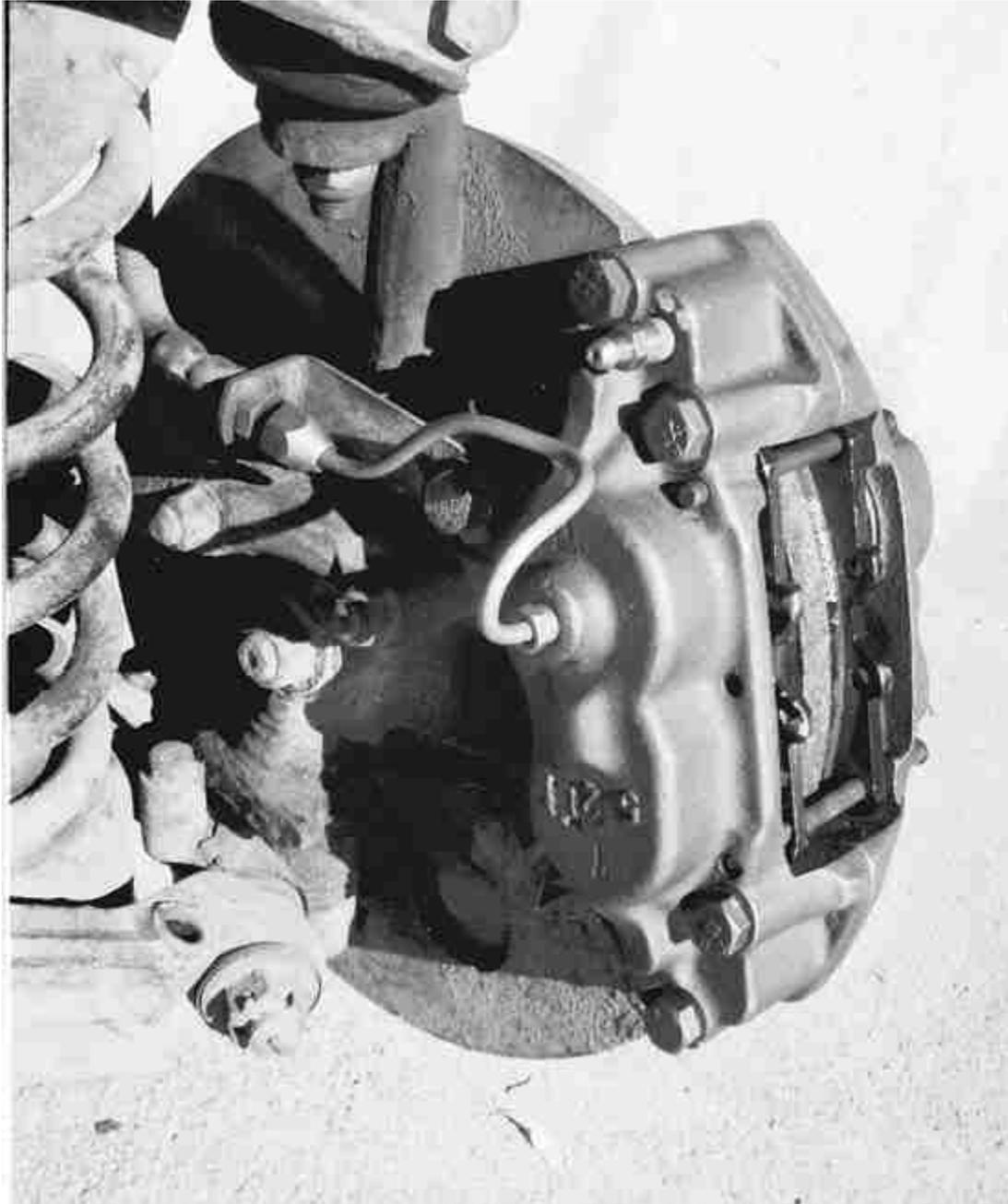
This is a photo of Toyota 1979-83 four wheel drive pickup (non-diesel) front caliper installed on a TR6 front axle. Note the hard brake line makes several bends to make it possible to access the caliper bolt without removing the brake line.
