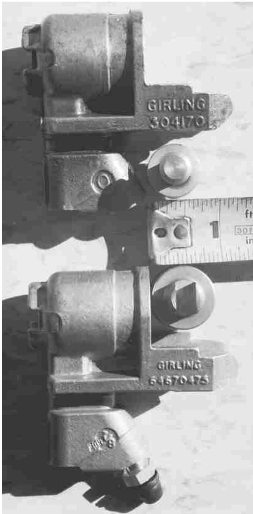
The top cylinder with casting number 304170 is a 0.70 inch cylinder for a TR6. The lower cylinder with casting number 64670475 is a 0.875 inch cylinder. for all Morgans from 1959 - 1988 (+4, 4/4, +8) and Sunbeam Alpine series 1 & 2.
