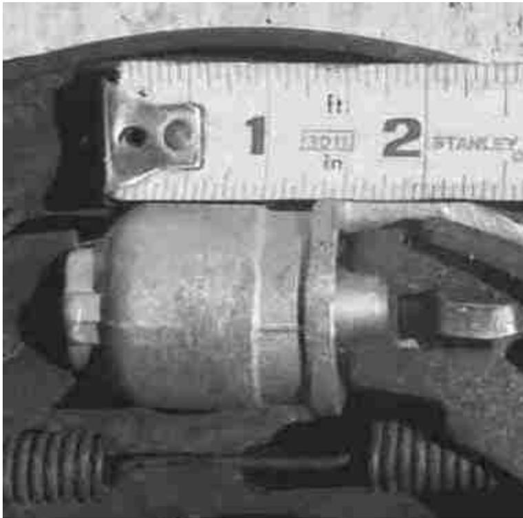
This is a photo of an installed Morgan cylinder. The major difference (other than the size of the cylinder) is the retaining tangs that help engage the brake shoe. Note that the tangs do not change the shoe position they simply limit lateral motion.
