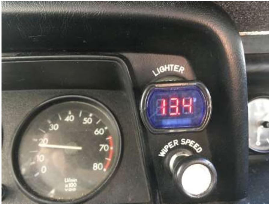
Verifying charging voltage – confirmation that the alternator is working properly – from the comfort of the driver’s seat with a cigarette lighter voltmeter.
