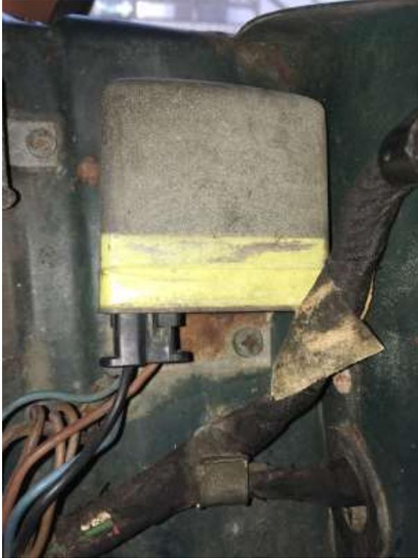
The three wires connecting the external regulator to the alternator are a common source of failure on a vintage car.
