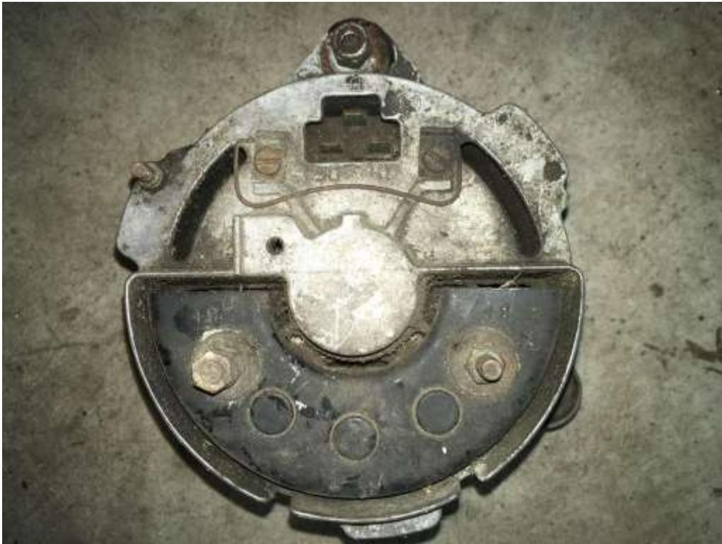
The back of a 1970s era Bosch alternator with its battery (B+) and regulator (D+, D-, and DF) connections.
