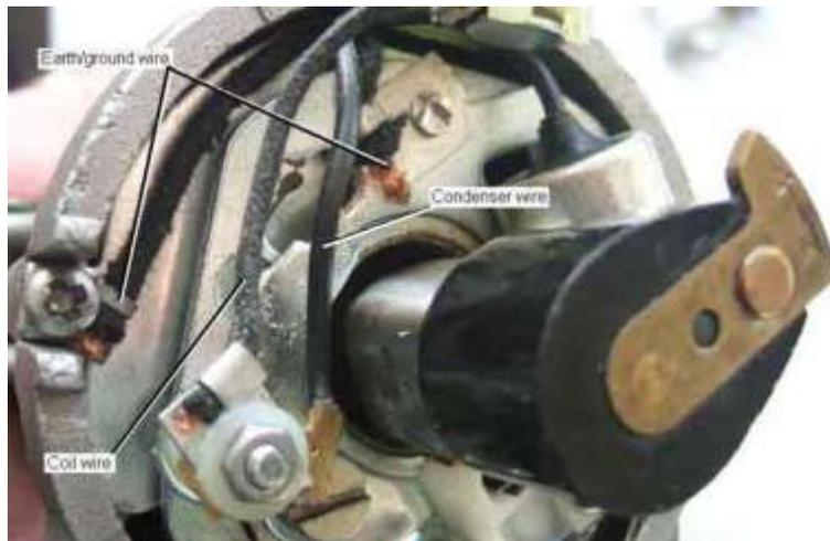
The condenser for the 25D distributor, that for the 35D8 for the V8 is very similar:
