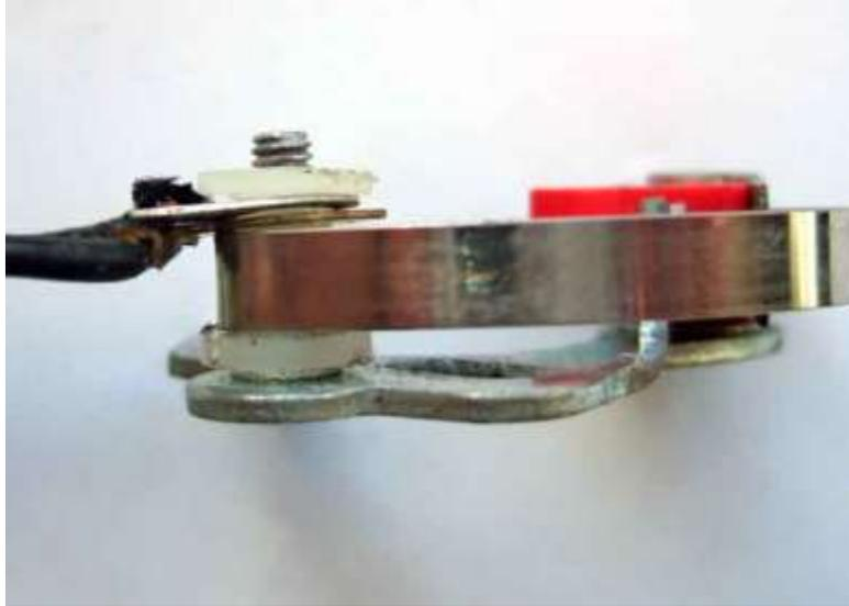
Finally the nut. These seem to be 'handed' in that one side seems flat and the other side has slightly rounded edges to each flat of the hexagon. I always put the flat side against the upper insulating washer as it just seems more 'correct', but I don't suppose it is critical.
