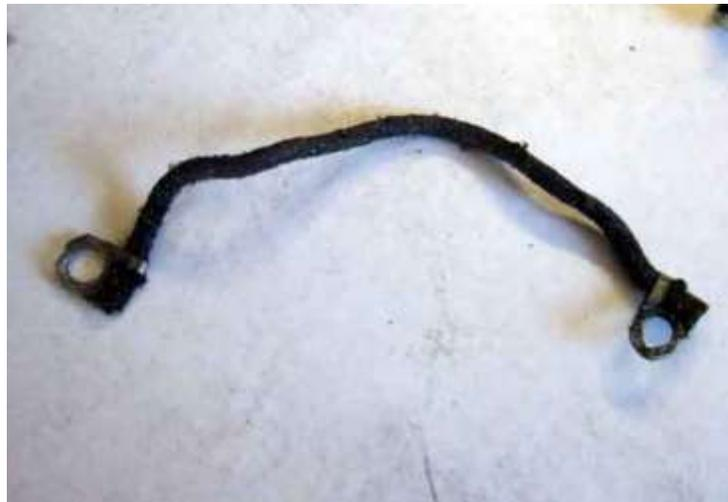
45D cloth-insulated earth/ground wire fitted, under the condenser fixing screw (condenser removed for clarity) and points plate fixing screw:
