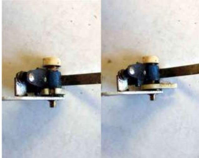
The connection arrangements are the same for both fixed and sliding types, however note that they are **not** interchangeable as the two base-plates are different. The sliding type have a small peg on the points and a locating hole in the base-plate (left), the fixed type have a large location peg on the base plate and a hole in the pivot, similar to the 25D type shown here on the right:
