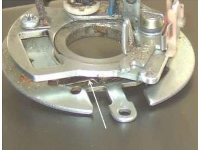
Cloth-insulated earth/ground wire for a 45D, screw tags at both ends, so can be replaced independently. This could be used as a replacement for the 25D as well, if obtainable:
