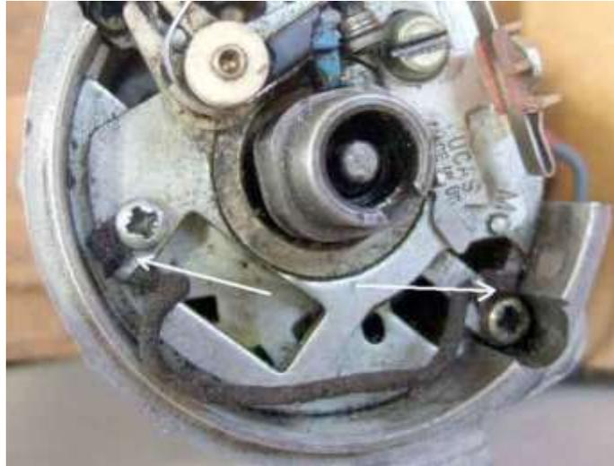
Combined condenser, coil wire and connection tag for the 45D distributor:
