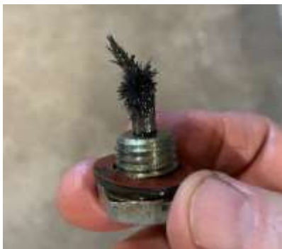
Picture 1. Excess metal on drain plug magnet.
