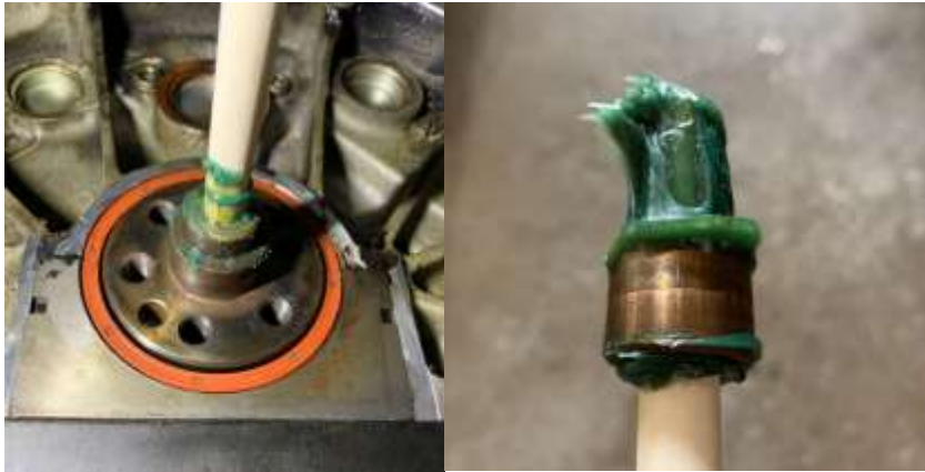
Pictures 7 and 8. Using grease to remove pilot bushing.
