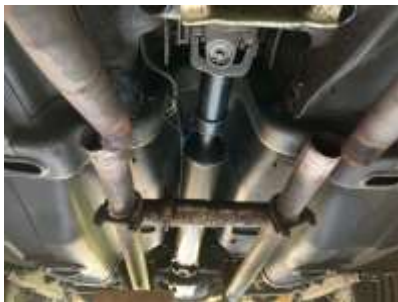
Picture 4. Exhaust finally apart.
