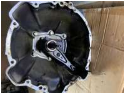
Picture 5. Oil inside bell housing.
