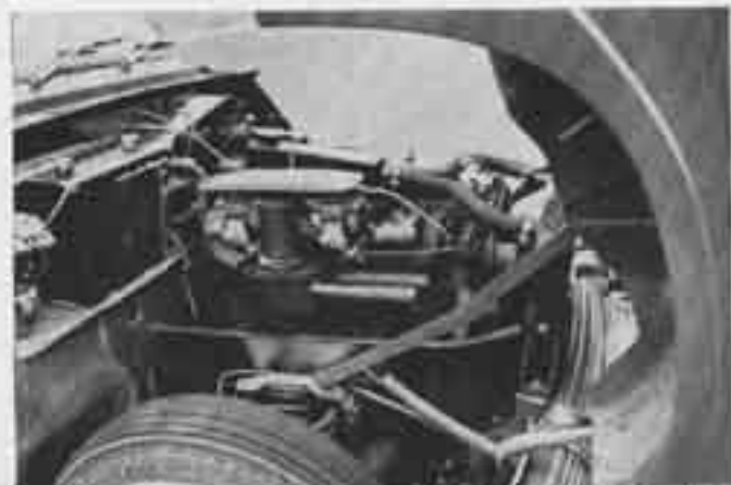
Low and narrow downflow-type radiator has small header tank mounted above the intake manifold to get it high enough.
