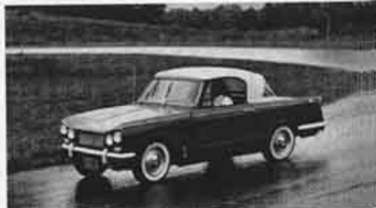
Cornering behavior of the Sports Six is good and the swing-axle rear suspension's inherent oversteer is not a problem.
