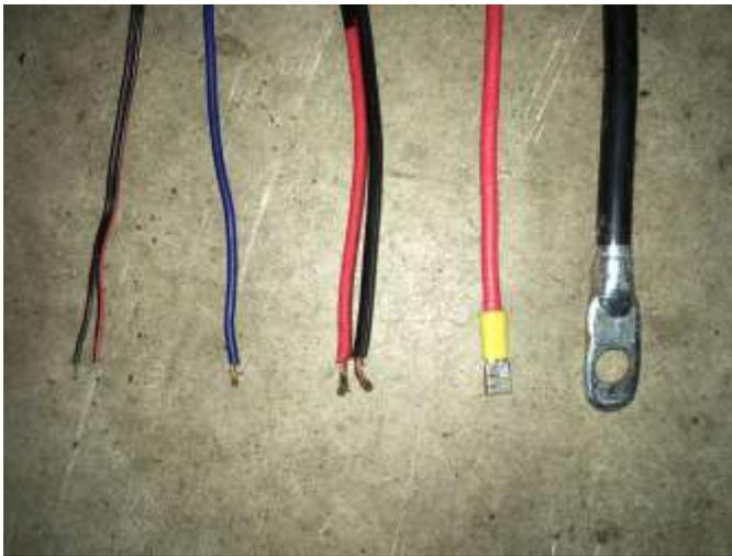
*Wire sizes from a 2 gauge battery cable (right) to 20 gauge speaker wire (left). Each has its place.*
