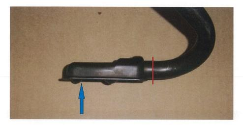
Above: the blue arrow indicates the opening on the Dodge part. The red line is where the tube will need to be cut (it is slightly expanded there to yield the 19mm ID). Sand the interior of the pickup tube opening and the exterior of the Triumph tube. They will need to be very clean for soldering. Check to ensure that the parts will slip together.
