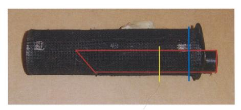
The image below shows the Triumph tube outline superimposed on the Dodge part. It is important that the relative positioning of the slash cut Triumph opening is the same as with the Dodge part (oval opening underneath). The opening is relatively centered over the Triumph oil pan floor. The Triumph tube will need to be cut at approximately the yellow mark. Measure twice, cut once!
