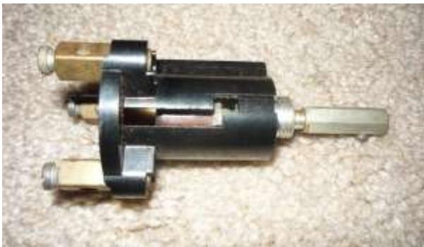
**Photo 7:** Forward tab on later switch; note there is no rear tab.
