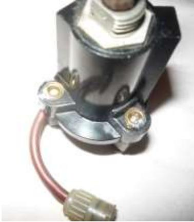
**Photo 4:** Solder for inner contacts and wire added for fuse.
