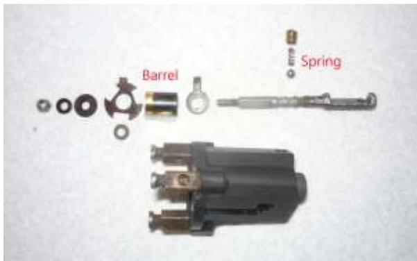
**Photo 1:** Pay particular attention to the small spring and ball bearing.
