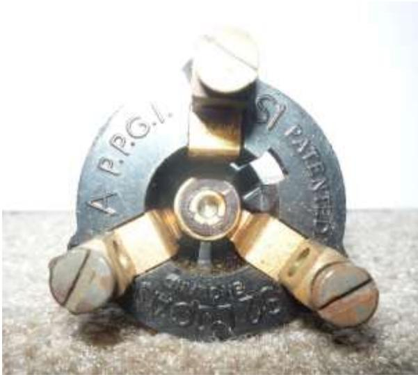
**Photo 6:** NOS Lucas 31126 replacement switch, which is riveted together.
