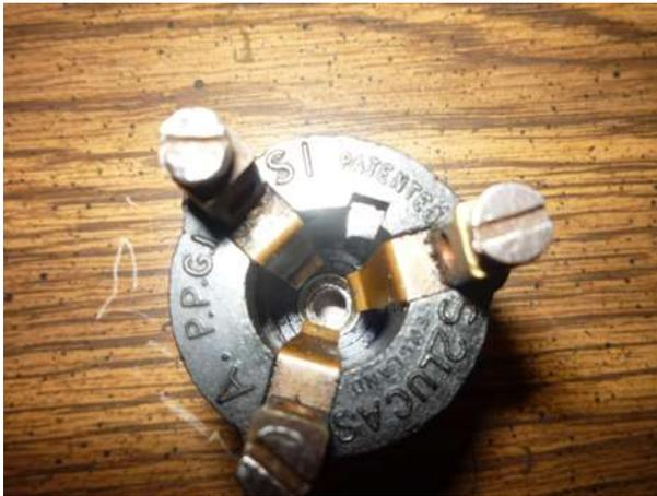
**Photo 2:** The inside of the switch and the contact fingers.
