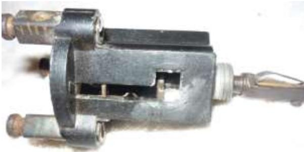
**Photo 5:** Groove repaired with JB Weld to provide Side light stop.
