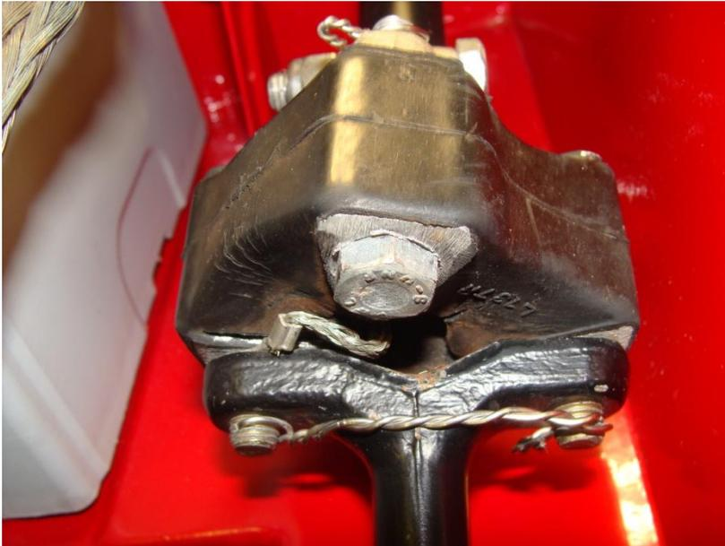
The jumper strap bonds the lower steering column to the upper column.
