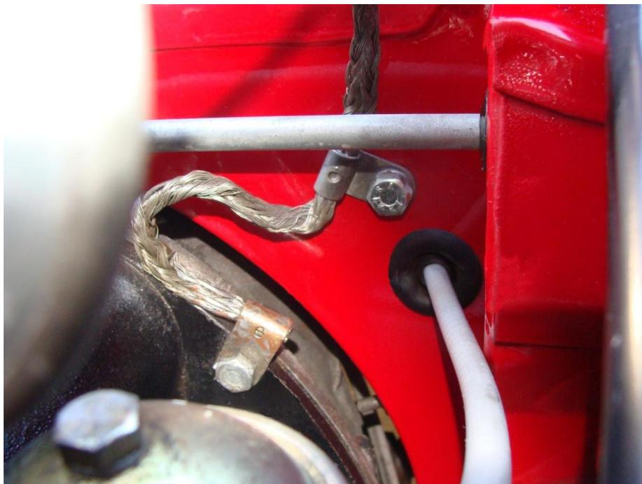
The Battery Ground Cable connects to both the Body Tub and the engine block.
