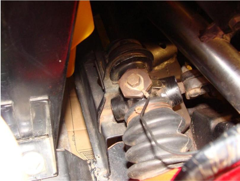
The wire drops down from the front harness running along the LH wheel arch.
