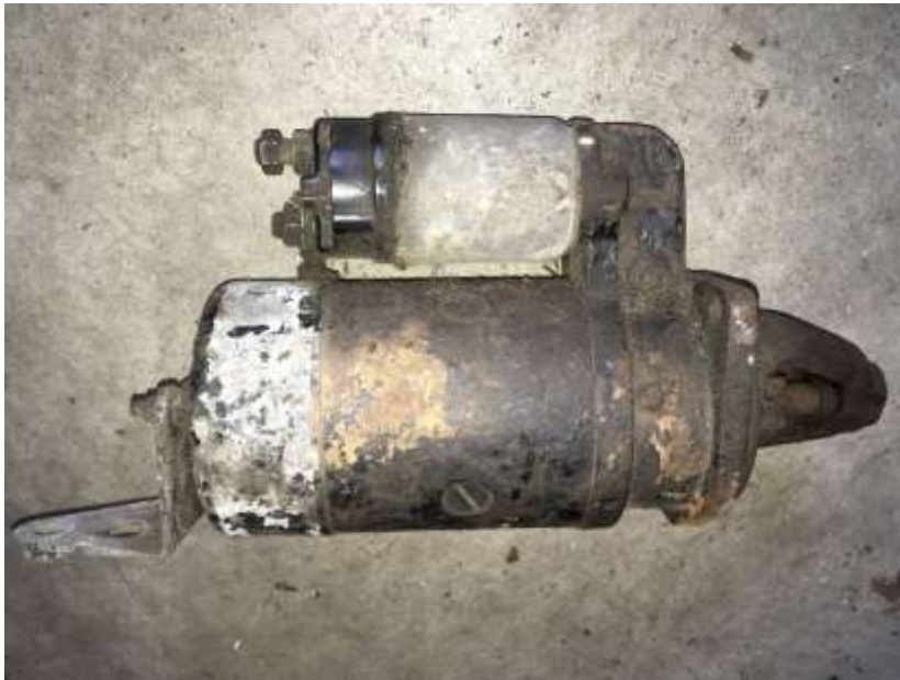
The starter and solenoid. On most cars, they're a tightly-coupled unit.
