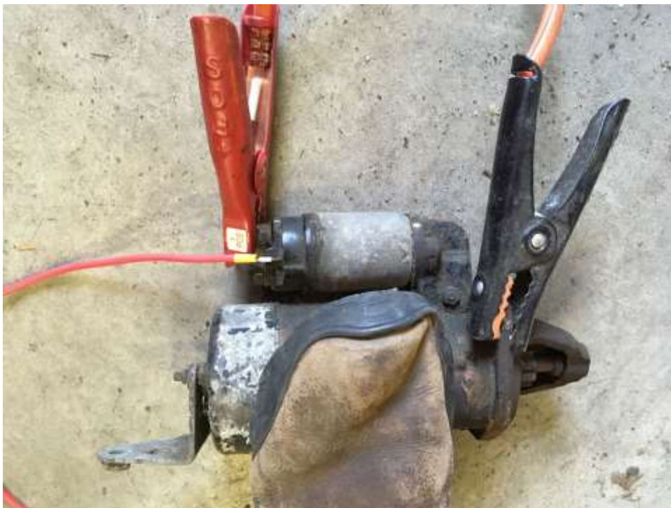
Testing a starter on the floor. Don't forget to stand on it or it'll jump dangerously around.
