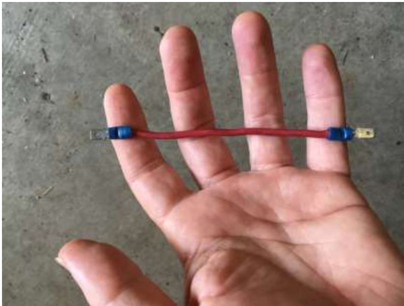
The legendary and ubiquitous jumper used to bypass a relay. Rob Siegel
