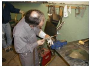
point. The tools were a sand-filled leather 'pillow' and a plastic/urethane hammer custom ground to the right shape. In a matter of a few minutes this flat steel was a dimpled bowl. Robin then took the piece-in-progress over to the English wheel and after a few minutes pushing and pulling the dimples were out and the bowl was super smooth.
