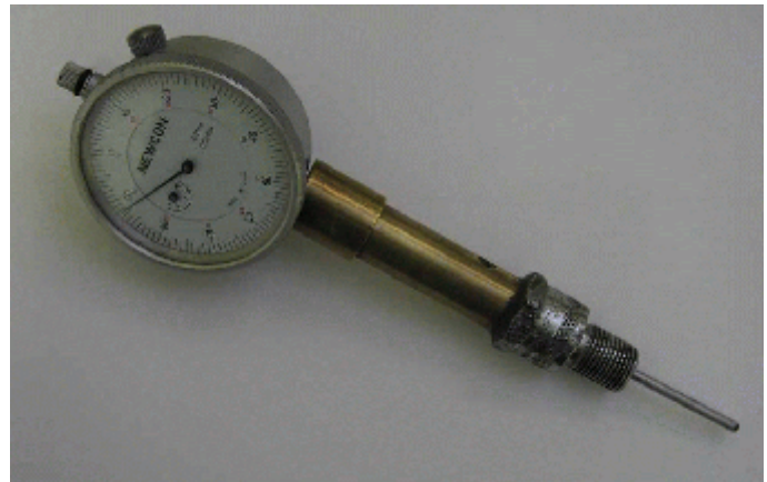
Figure 1. Gauge (on right) used to determine TDC of cylinder one. Here I am working on Bob Thomas' TR6.
