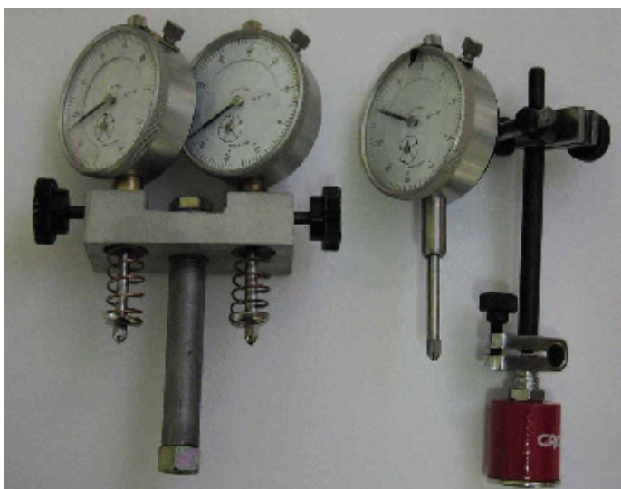
Figure 3. Gauges (on left) used to measure the crossover point of the valves. Gauge on right is used to determine TDC when the head is off (magnetic base holds it to the block).
