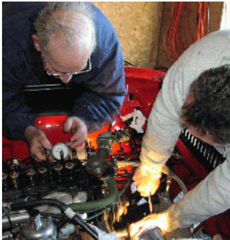
Figure 1. Gauge (on right) used to determine TDC of cylinder one. Here I am working on Bob Thomas' TR6.
