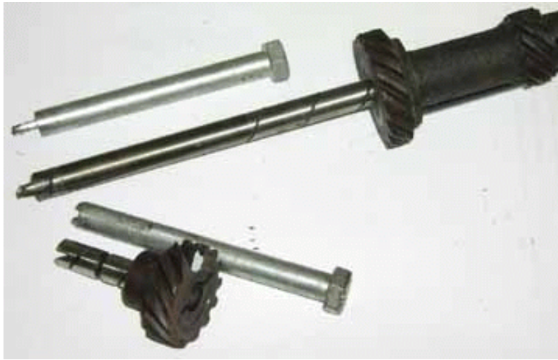
Figure 4. The distributor gears from a TR4 (top) and TR6 (bottom) with the modified bolts used to position the oil pump. Note the white dot on the TR6 gear to help reduce confusion when trying to align the gear.
