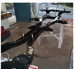
worried the paint would be too thick on the chassis. Now, to avoid messing up the paint when we flipped the frame, we used some bolts and piping. The bolts went on the topside near the rear of the frame, and the tubes fitted over the underside rear diff mounts. The results speak and shine for themselves, but that's sort of where my progress slows.
