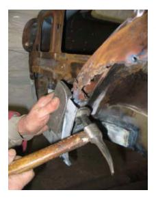
In order to fabricate new pieces into the panel, we first cut some templates from card board [ for additional help taking measurements from our MK3 Spitfire] and fitted this template to the wheel housing. After we were satisfied with a proper fit, we proceeded to cut the replacement piece out of sheet metal.
