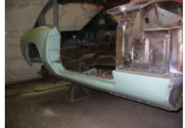
seams. Next job on the list was the application of a layer of body filler and, after drying, sanded it with 40 grid, followed by a second sanding of 80 grid, making sure that the contours of the panel were retained and the panel was straight, confirming to originality. In order to obtain this, one may have
