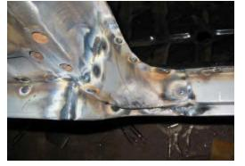
The welds had been ground off, using a 36 grid, flexible disk on a small air powered grinder.
