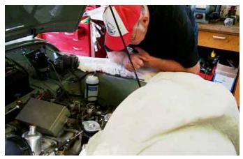
Gapping the pushrod/rocker arm takes only a few minutes and we bolt on the valve. I worked really hard during that process. I was the one designated to turn the engine at top dead center while Brian and Roly
