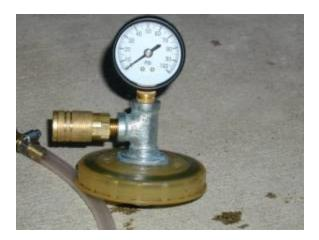
Next, you will need a spare cap off of an old master cylinder. Bore a hole in the center, use some blue silicon sealer to be sure you are airtight. Attach a standard pressure gauge to the t connecter, use a quick connect on the other side. You get something like this:
