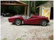
ReBuilt to TR3B spec. Body Off ,to bare metal, epoxy primed & Epoxy undercoated. Marine grade stainless steel fasteners, new elec wires, and seals, etc.. Engine rebuilt to TR3B spec. full synchro TR4 trans., stainless steel Monza exhaust, Hayden electric fan, New top, leather seats, 60 spoke wheels, SOLID CAR Sandy Stewart Caledon East 905-584-2941 <u>arielcyclone@hotmail.com</u> [1]
