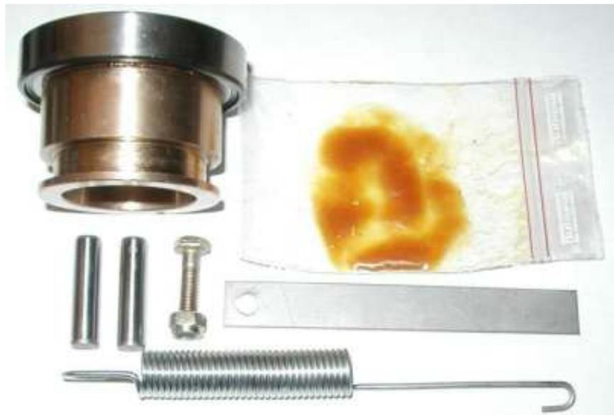
**Important!** Prior to installation make sure the two dowels between the engine plate and the gearbox are present. Missing dowels can cause rough jerky clutch operation as the release bearing is not centric to the clutch (See drawing)
