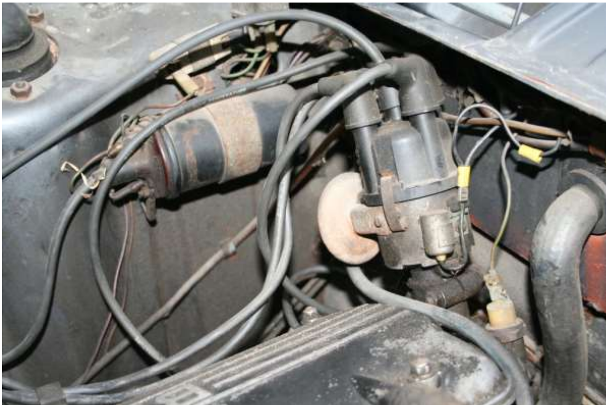
Distributor and coil on a 1973 BMW 2002tii.
