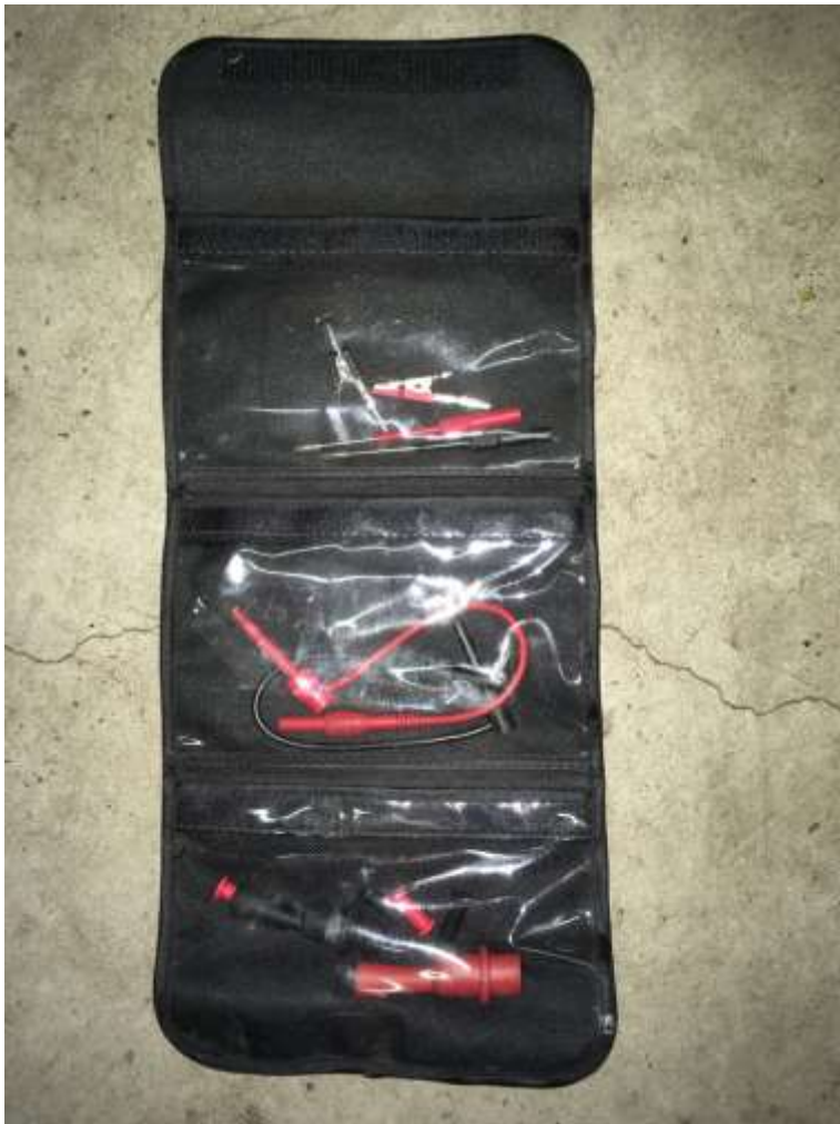
An inexpensive set of probe lead attachments.
