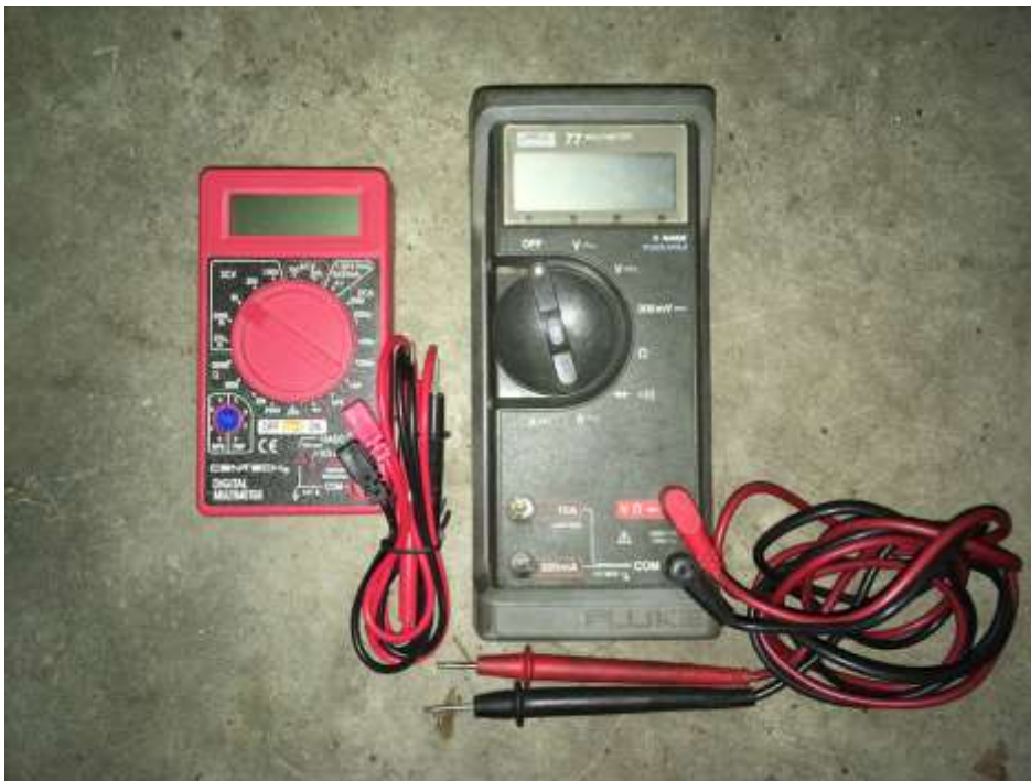
The Harbor Freight $5.99 multimeter (left) does not have autoranging, and consequently, its center selection dial is cluttered with options. In contrast, any autoranging multimeter (right) has a much simpler dial.
