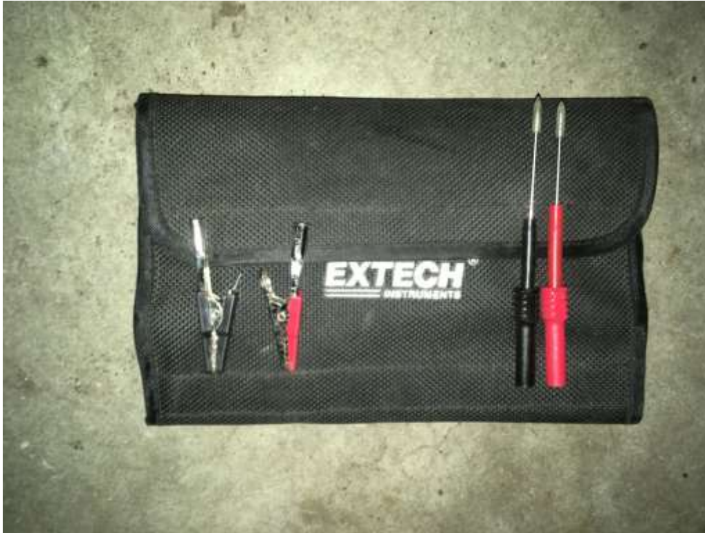
The two most useful probe lead attachments: Alligator clips and back-probe pins.
