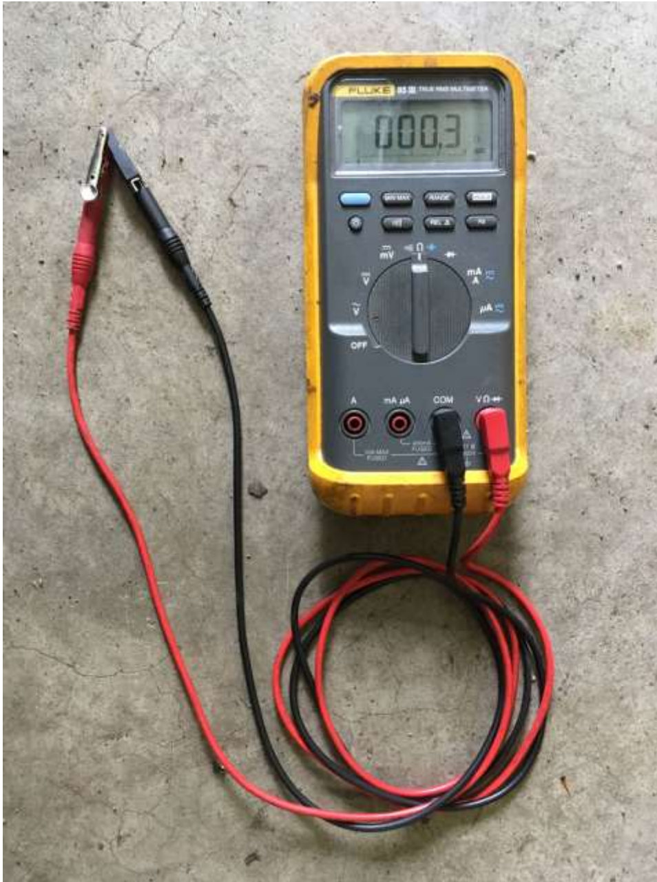
The sub-one-ohm reading indicating continuity
