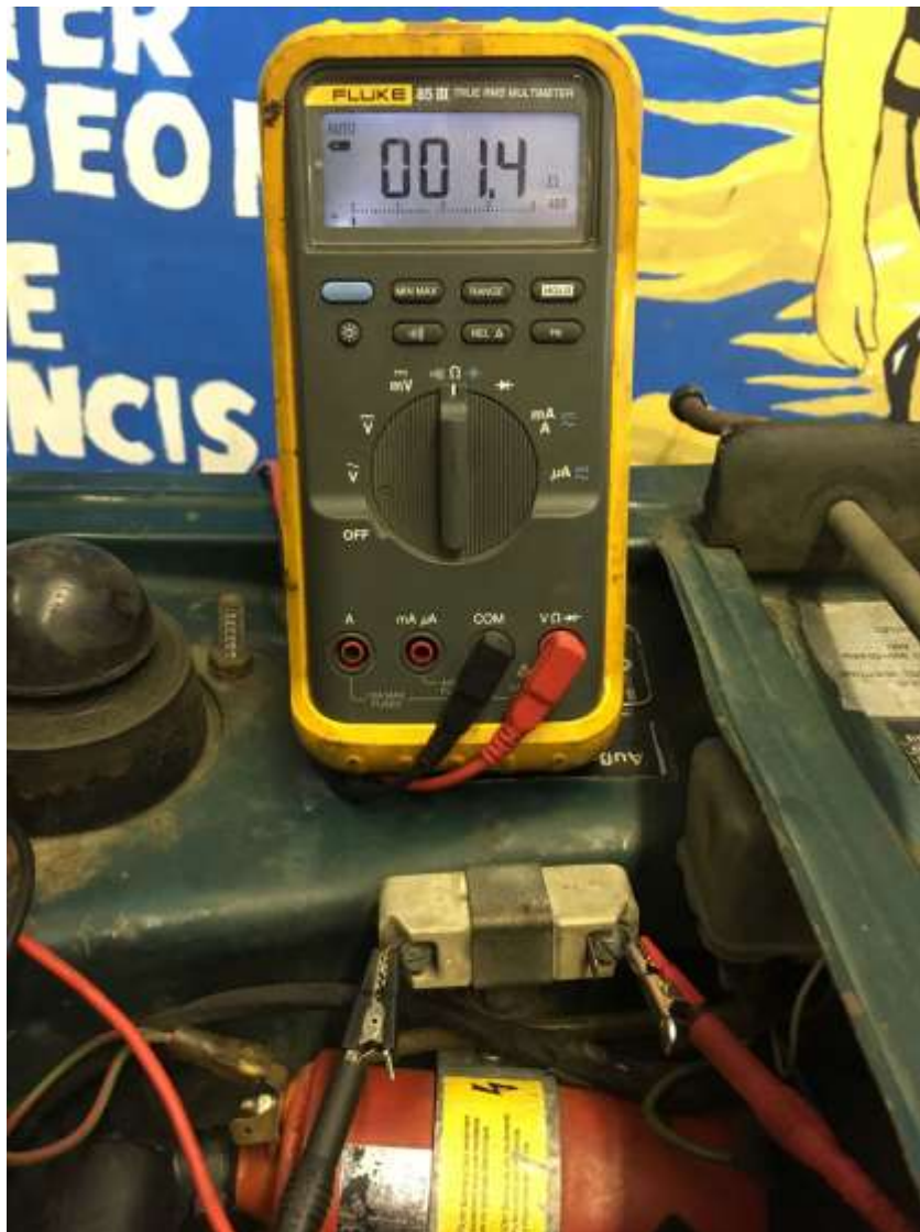
The resistance of this ignition coil is 1.3 ohms
