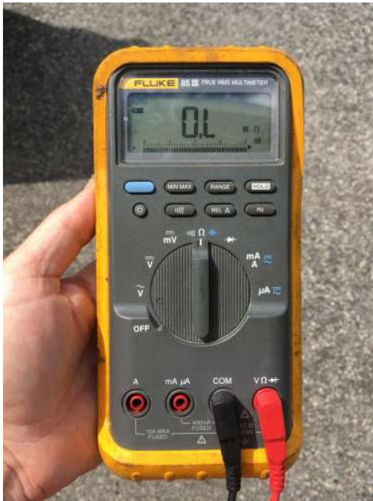
A multimeter configured to measure resistance (red probe in the “V \Omega ” socket, rotary dial turned to the resistance setting)
