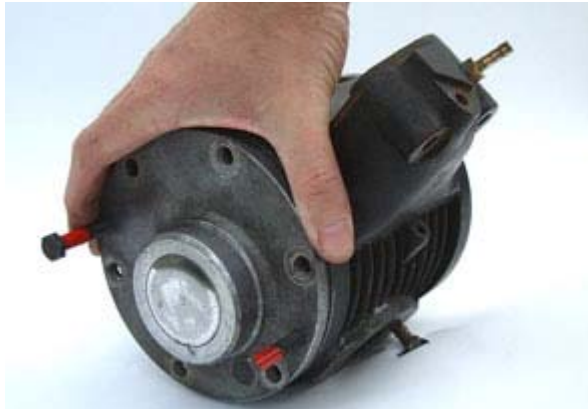
2. Use two 5/16th USS bolts to remove rear cover The main bearing fits snugly into the front housing
