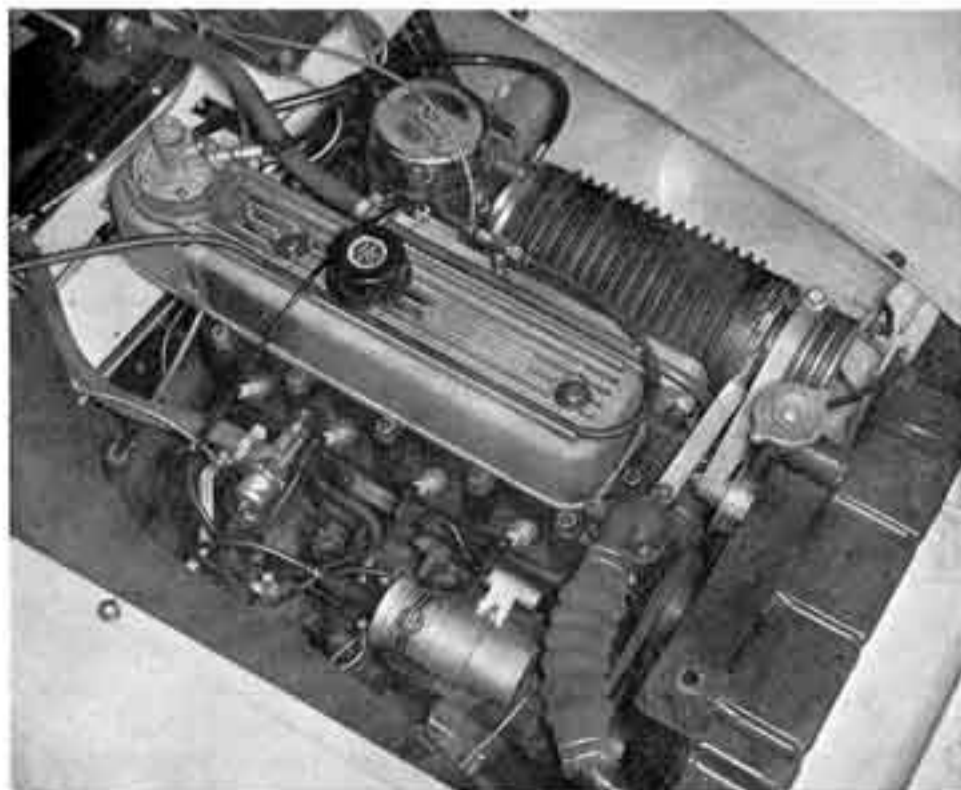
No alteration of panel was necessary to install blower.
