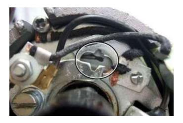
The fine adjustment 'V-notch and pip' (circled) of 45D sliding points (45D fixed points have the V-notch at the pivot end of the points plate):
