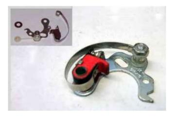
First on the threaded stud is a stepped insulating washer, with the step facing upwards.
