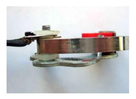
Finally the nut. These seem to be 'handed' in that one side seems flat and the other side has slightly rounded edges to each flat of the hexagon. I always put the flat side against the upper insulating washer as it just seems more 'correct', but I don't suppose it is critical.
