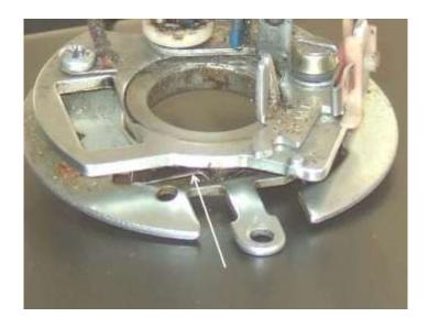
Cloth-insulated earth/ground wire for a 45D, screw tags at both ends, so can be replaced independently. This could be used as a replacement for the 25D as well, if obtainable:
