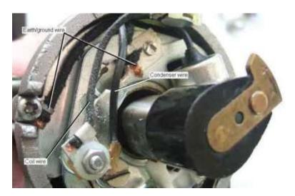
The condenser for the 25D distributor, that for the 35D8 for the V8 is very similar:
