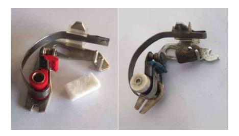
With this type the moving contact spring just lays in a channel in a plastic insulator fixed to a post on the fixed contact base. The end of the spring has a partially flattened loop, and a flat brass connector with the condenser and coil wires already attached simply slides into the loop. The only important thing here is that the plastic insulator does lie between the post and the spring.
