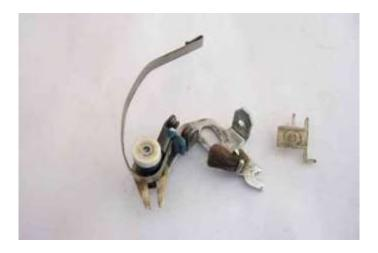
Showing the 45D 'sliding contact' type, with the points plate in the minimum vacuum advance position on the left and the maximum vacuum advance position on the right. Note the difference in angle of the slotted lever (circled):
