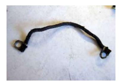
45D cloth-insulated earth/ground wire fitted, under the condenser fixing screw (condenser removed for clarity) and points plate fixing screw:
