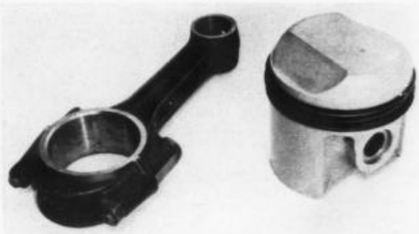
Connecting rod, with as-forged finish, has deep webbing on the big-end cap. Piston is slipper-type, having a skirt on thrust faces only.
