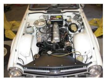
Despite the imposing 46-page instruction manual and the number of parts included in the box, the installation is quite simple. First, the radiator, front chassis crossmember and pulley system need to be removed. The intake manifold and carbs are then pulled from the engine.
