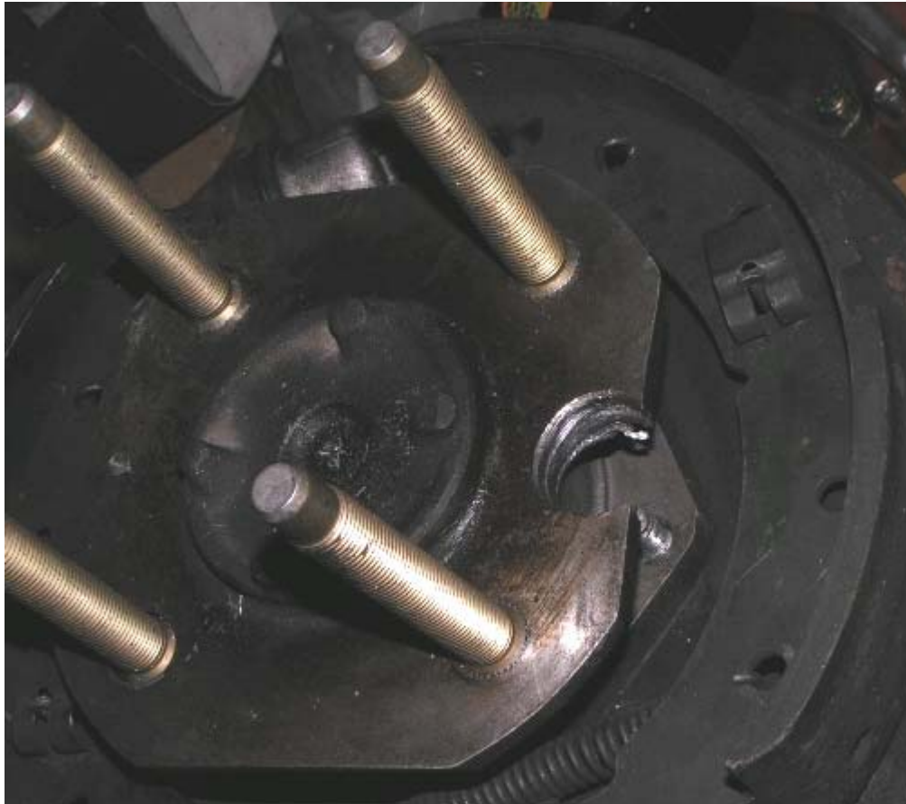
Figure 14: Hole Drilled in Nissan Axel Flange
