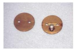
Comparison of earlier- and later-style throttle disks shows that the later-style disks have a spring-loaded poppet valve, which impedes air flow. Replace these with earlier-style disks in performance There are not too many performance modifications necessary or possible for SUs. Aside from changing to larger carbs, about all that can be done is to change to needles with a different taper and make modifications to increase air flow around the throttle disk and shaft.
