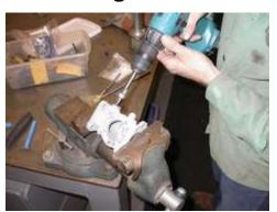
Replacing the throttle shaft bushings requires reaming out the old bushings, installing new bushings, and reaming the new bushings to size.
