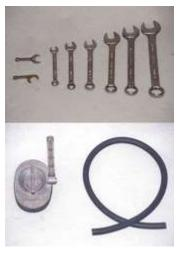
A set of British wrenches and SU jet wrenches (top) are useful tools when working with SU carburetors. These are available from most British car suppliers for relatively low cost.
