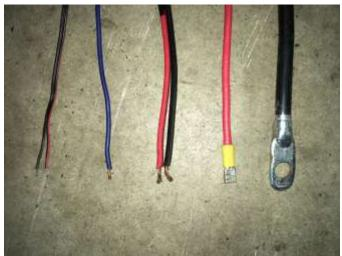
Wire sizes from a 2 gauge battery cable (right) to 20 gauge speaker wire (left). Each has its place.
