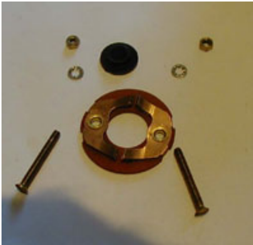
The components just removed (including the button that retains the horn push spring)
