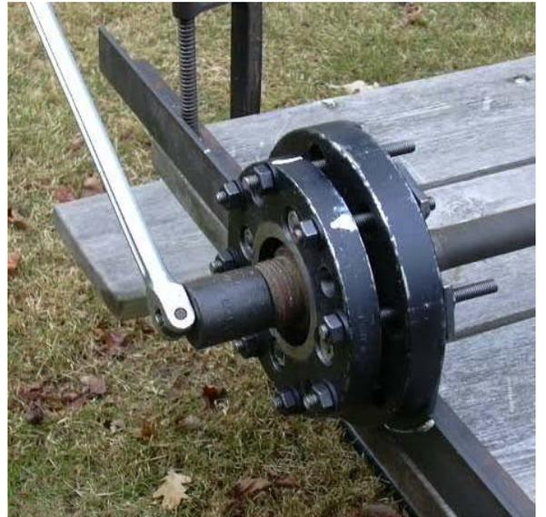
Arrange the assembly on the nearest picnic table as shown. Back the nut off so that it is flush with the end of the axle.
