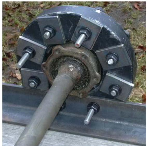
Use the angle iron to bolt the assembly to the nearest picnic table. Remove the axle cotter pin and loosen the axle nut (1-1/4" socket).
