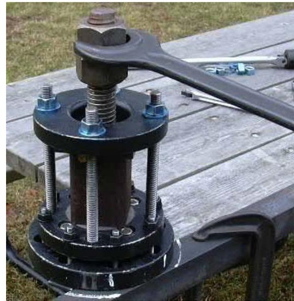
So now we need to get the bearing off of the axle shaft. Rearrange the pulling plate, and the Acme nut stop to the pictured arrangement. Now we see why the hole in the Acme nut stop was bored to a diameter of 1.765". This is the diameter needed to just clear the shoulder on the axle and allows contact with the bearing. It is assumed that the bearing will not be reused.
