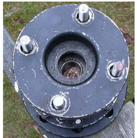
Put the nuts on the 4 threaded rods and check that the rod is fully threaded into the nuts in the counterbores. Don't tighten at this time. Install the 1-1/2" Acme pressure screw with the double nuts into the nut captured within the square tubing. Make sure the 4 threaded rods are fully engaged in lower nuts and then tighten the 4 nuts to 120 ft-lbs (15/16" socket) progressively in a star pattern
