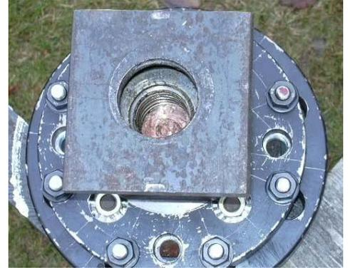
Screw the 5/8" grade B7 threaded rods into the shortened nuts that were placed into the counterbores of the puller plate at the beginning of the puller assembly.
