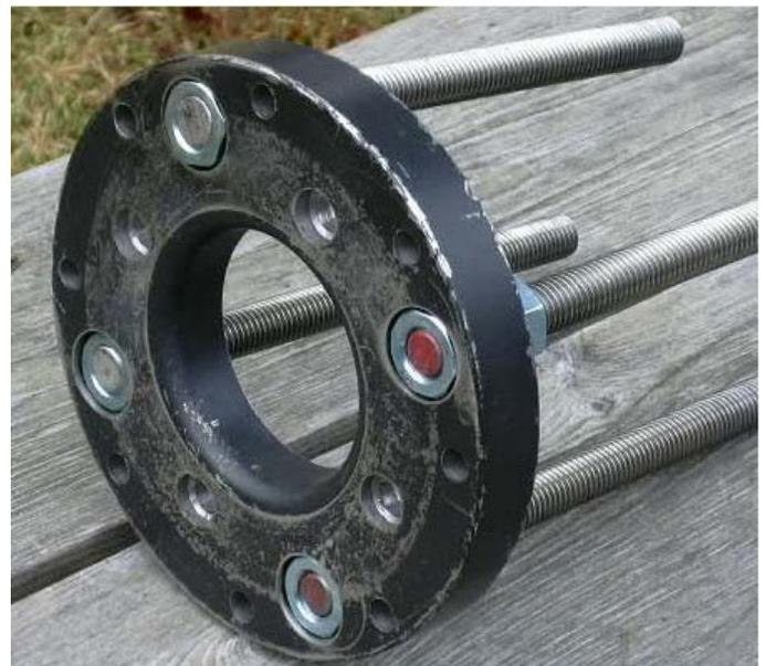
Now we are ready to assemble the pulling plate to the hub/axle assembly. Place the shortened 5/8" grade 8 nuts into the counterbored holes of the pulling plate. These are grade 8 nuts that were slightly faced down on the lathe to fit the counterbore depth of the pulling plate. The plate is then bolted to the hub wheel studs using grade 8 nuts and tightened to 55 ft-lbs torque (11/16" socket)
