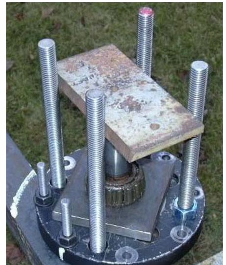
Place the round strongback on top of the plate strongback, install the nuts and tighten the nuts a couple turns at a time progressively until the bearing is free of the axle.
