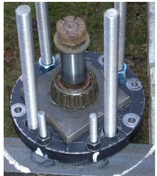
With the nut flush with the end of the axle shaft place the copper softener on the nut.
