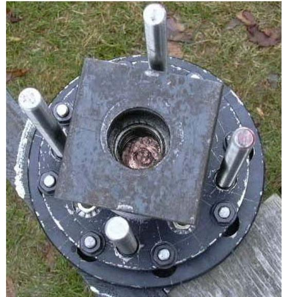
Place the round strongback onto the nut stop. This strongback is a 2-1/2" 150 pound raised face flange.
