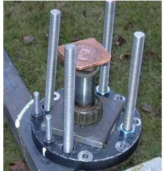
Place a steel plate strongback on top of the softener.
