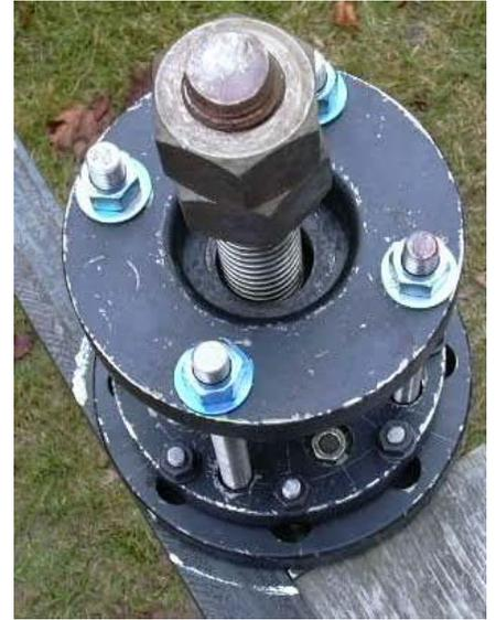
Using your standard 60mm or 2-3/8" open-end wrench, turn the top double nut to tighten the pressure screw. Once there is resistance a few raps with a hammer on top of the screw should pop the axle out of the hub. The only indication that the hub is free from the axle is when the Acme screw loses tension. No loud noises or assembly jumping off the picnic table
