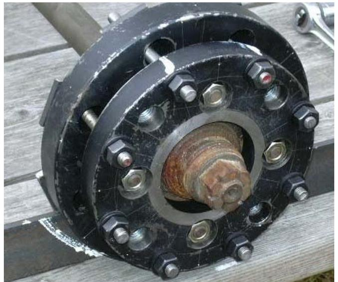
This shows a rear view of the assembly. The steel plates are used under the nuts to help spread the nut loading out over a wide surface on the flange.
