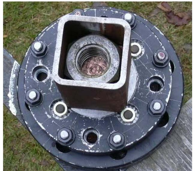
Install the stop for the Acme nut over the top of the square tubing. Note that the hole bored in the square plate is 1.765" diameter, which is useful later in the project.
