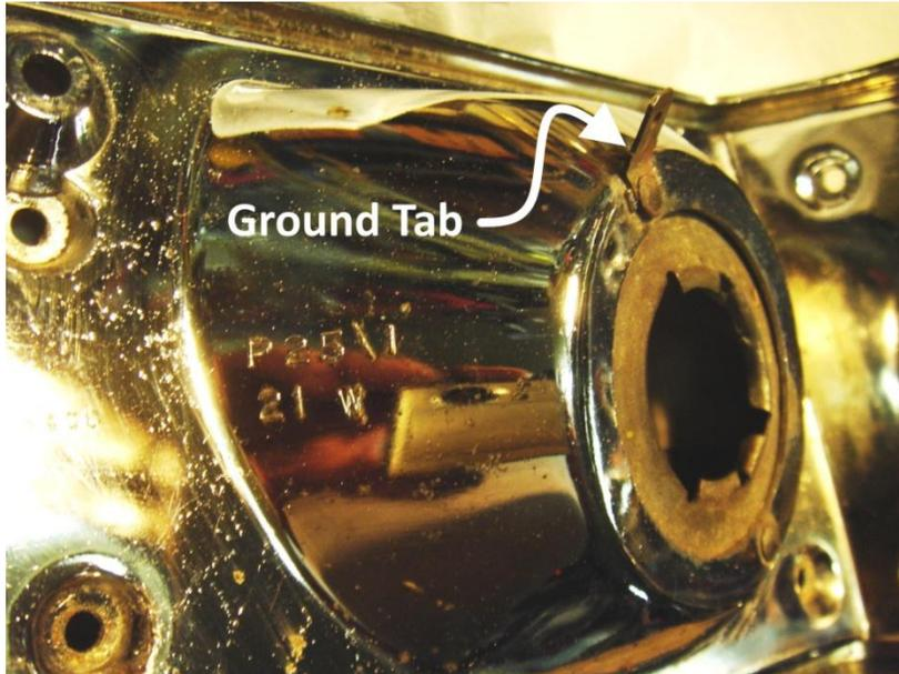
A black ground wire from the rear harness attaches to the ground tab at the turn signal bulb reflector of each taillight frame.
