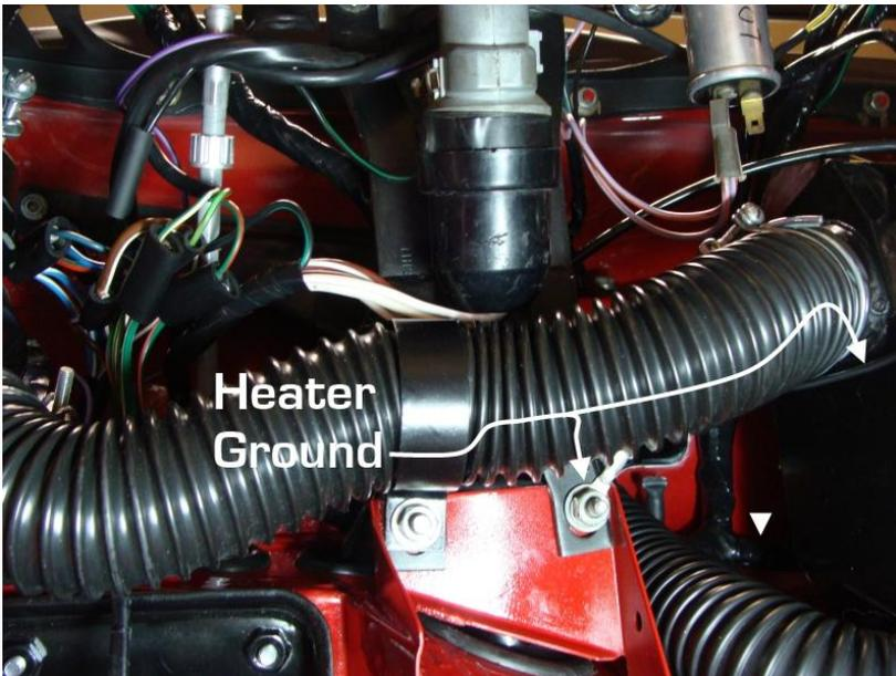
Early car heater motors have two white wires with one of them exiting the heater case as the ground wire along with the low and high speed wires.
