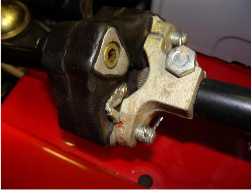
The strap routes through the hole in the flexible coupling.
