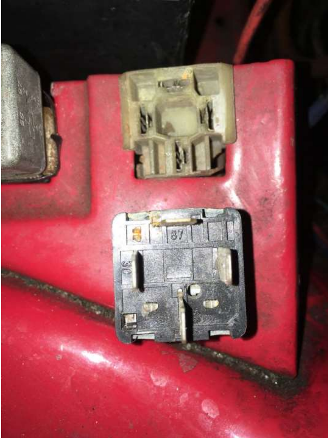
Relay removed from its socket, showing the DIN numbers on the bottom. Rob Siegel
