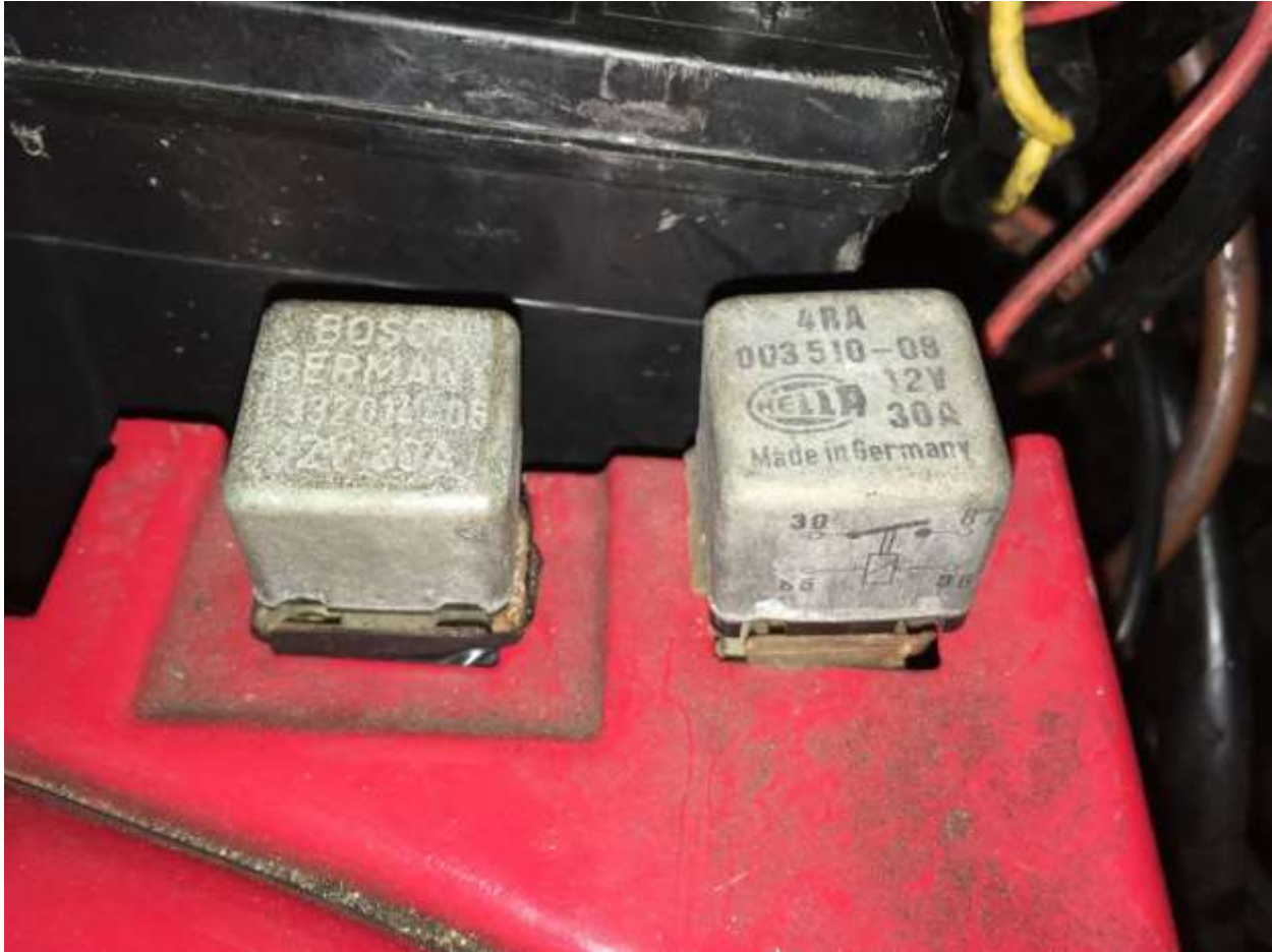
Two DIN relays in an early '70s German car. They've changed very little since then. Rob Siegel
